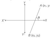
The slope of a line *AB* is  $m = \tan \theta = \frac{y_2 - y_1}{x_2 - x_1}$
